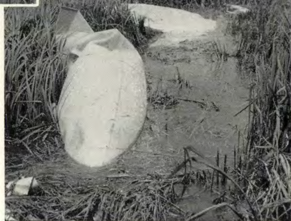
The pilot undershot the runway and hit a rice field. The wing tiptank broke off as the plane struck several small dikes. There was no fire or explosion.
