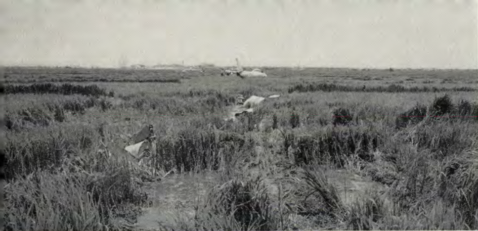
The pilot undershot the runway and hit a rice field. The wing tiptank broke off as the plane struck several small dikes. There was no fire or explosion.
