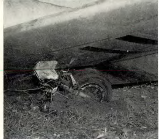
The aircraft contacted soft ground of a turnip patch at minimum flying speed, coming to a stop after skidding 216 feet. Leaving the gear down allowed the pilot to land in a normal attitude.
