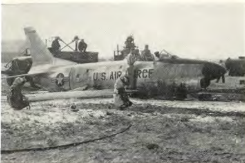
Structural damage, top photo, resulted when F-86 hit fire plug. Aircraft came to rest at a 90-degree angle to runway direction.
