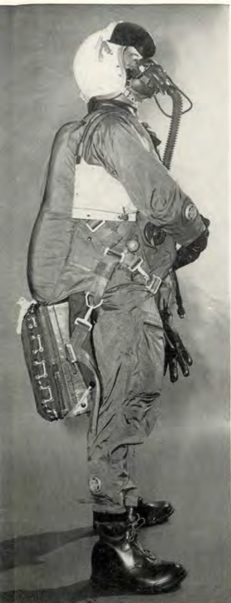
Left, pilot is wearing anti-exposure suit. Above shows underarm life preservers, back type parachute and the A-1 survival kit.
