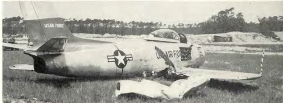
In another F-86 accident the gear absorbed the landing shock. Top photo shows the second impact with the ground when pilot undershot. The F-86 bounced 300 feet from point of first impact, skidded approximately 400 feet then veered to right.
