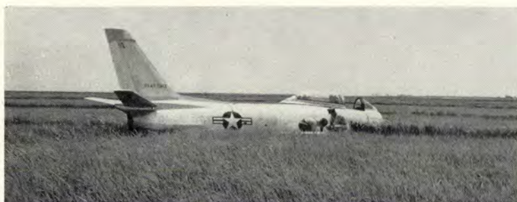
The pilot undershot the runway and hit a rice field. The wing tiptank broke off as the plane struck several small dikes. There was no fire or explosion.
