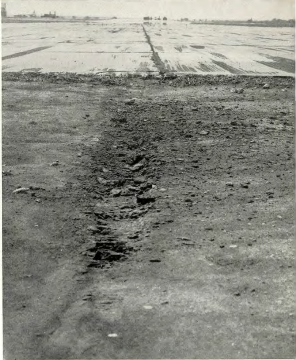
The landing gear will withstand a terrific impact. This F-84 touched down short of the runway; the tire exploded and the aircraft slid on the wheel hub for 4500 feet.
