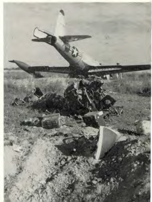
This T-33 went through fence and drainage ditch. Entire nose section was torn free. Pilot was uninjured. Gear absorbed shock.
